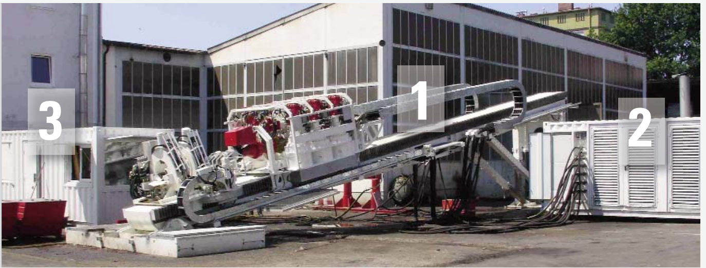
Rig, power pack & driller's cabin during commissioning
